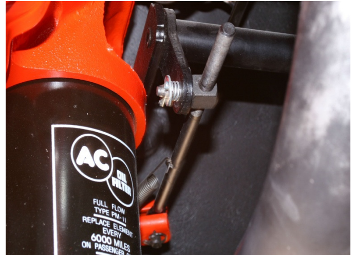
Picture 2-Clutch Fork, Pushrod, Swivel, and Inboard Cross Shaft Lever
