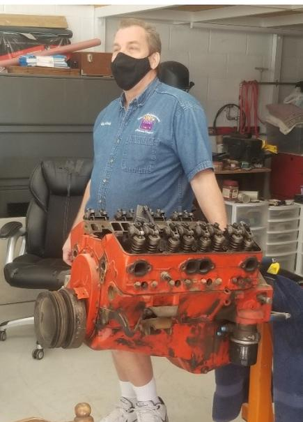
see an engine on a stand so the action of the cam, lifters, pushrods, rocker arms and valves could be seen relative to the crankshaft balancer.
