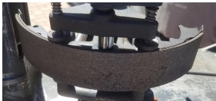
The picture at right shows how the shoe fit against the drum now that it has been arched to match up with the drum (minus the slight .030" CAM grind offset). The shoe pad is now much thinner as well.
