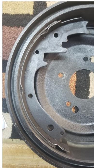
With this test completed, I felt comfortable with using the machine, and proceeded to re-arch the shoes on the wheel I took the drum off of. Took about .040" off each shoe to match the arch of the drum.
