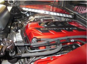
The check valve is pointed to the inlet port of the catch can. The outlet port hose is routed under the inlet hose and snapped into place. Over time, the hoses will heat soak and be more pliable for a nicer routing.
