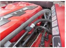
With a catch can, there is a check valve and it needs to be installed in the correct direction of flow. The arrow must point to the air plenum so the vacuum can pull the volatile gasses from the crankcase.
