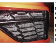
The front radiators get dented easily because they are near the road surface and they are a soft alloy. The race teams probably replaced them every other race, depending on the air flow loss. To avoid this expense, I recommend installing small mesh screens behind the factory grilles. Several vendors have these for sale, and the installation is not very difficult.
