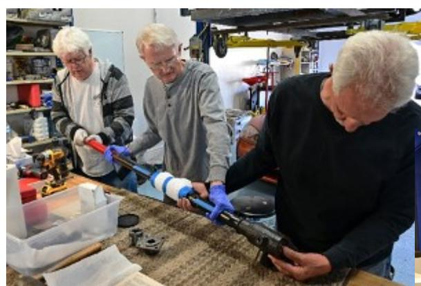
Mike and Garry compared measurements of the shaft resistance as John adjusted it to within factory specs. It was staked and then measured again to confirm that it was correctly set. [Note: detailed instructions for adjusting the steering box are provided in Reference (A); and alternative tools are identified in Reference (B).]
