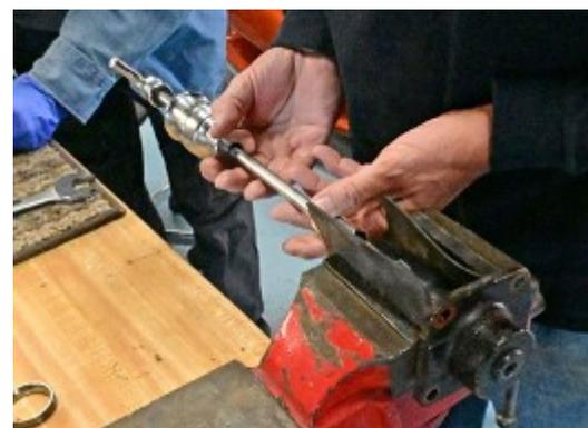
The new races were relatively easy to install with Garry's press. Garry uses a relatively low force and a series of gentle taps to seat each race. As shown in the photos, Garry used both press tools and large sockets. Note that the race for the upper worm gear/column bearing was not replaced as it did not appear to be worn – all of the wear was at the lower end.
